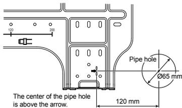
1. After determining the pipe hole position on the mounting plate (➔), drill the pipe hole (Ø65 mm) at a slight downward slant to the outdoor side.
