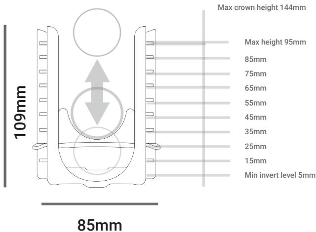
The Gel-clear APC19 is part of the bio-beta range of products for food retail refrigeration. A retrofit, adjustable pipe support for condensate drains running beneath chillers. Locks in place incremental slope settings. Statutory regulation requires a 19mm per metre slope on overground condensate drains.
