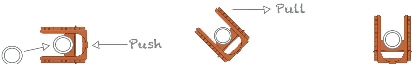
Fitted in seconds, the pipe support can be set at 10mm increments prior to fitting bringing BSEN12056 compliant sloping to flat drains.
